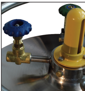
The Dura-Cyl LP models feature the "sight gauge" liquid level indicator and a liquid globe valve with an extended stem for less ice build-up on the handle for easier operation.
