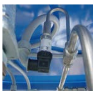
Integrated Bulk Tank Pressure Sensor
